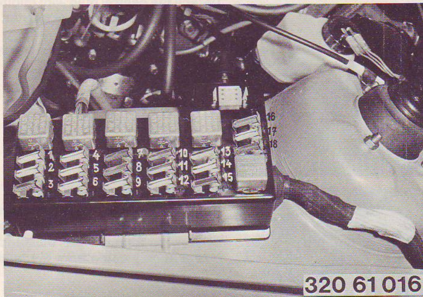
Arrangement of fuses
